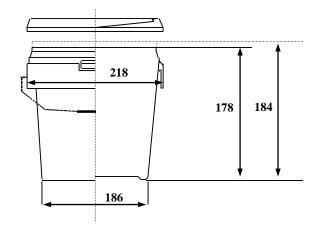
Measurements in millimetres
